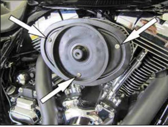
8. Install the K&N® air filter onto the back plate and secure with the provided hardware.
