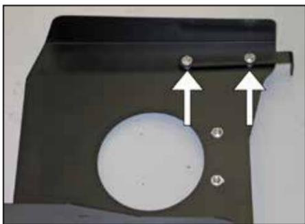
12. Install the heat shield mounting bracket (070902) onto the heat shield using the provided hardware and spacers as shown.
