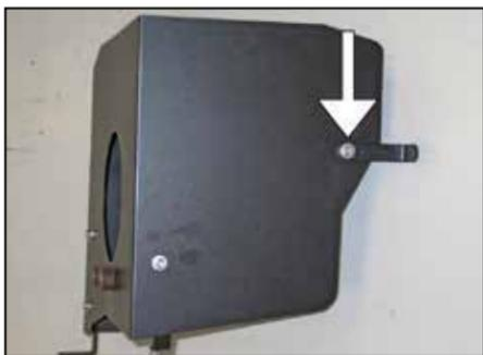
14. Install the provided heat shield mounting bracket (070742) onto the heat shield using the provided hardware and spacer as shown.
