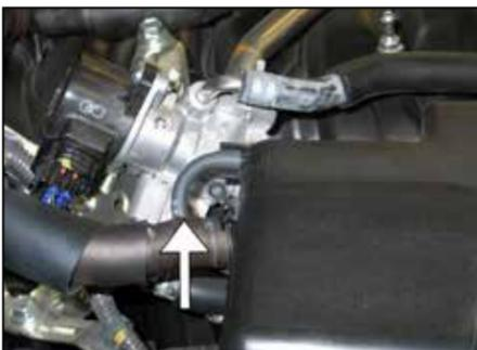
3. Disconnect the fuel pressure regulator vacuum hose from the intake tube.
