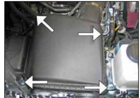
7. Release the four latches' securing the upper airbox to the lower airbox.
