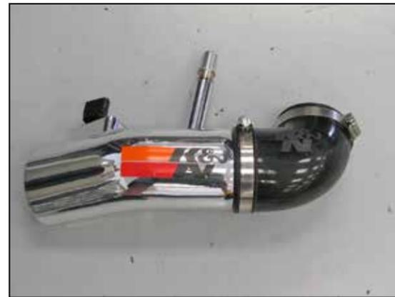
18. Install the provided angled coupling hose (084087) onto the intake tube as shown.
