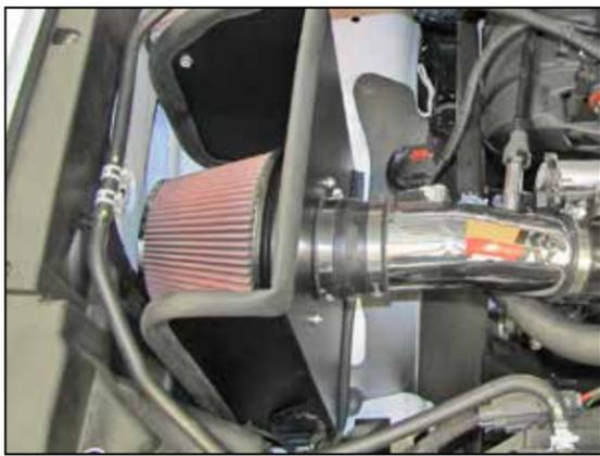
22. Install the K&N® air filter and secure with the provided hose clamp.
