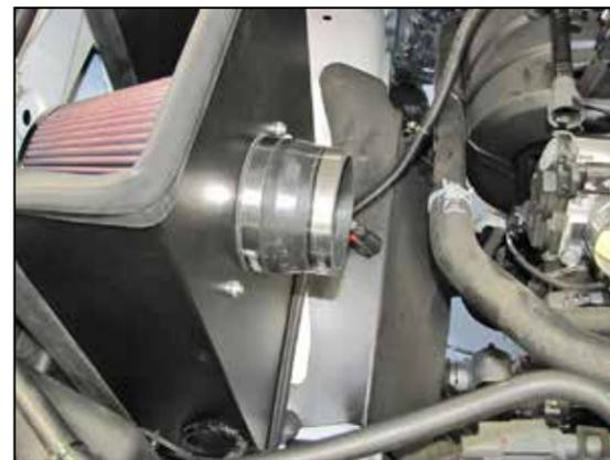
17. Install the provided coupling hose (08051) onto the filter adapter and secure with the provided hose clamp.
