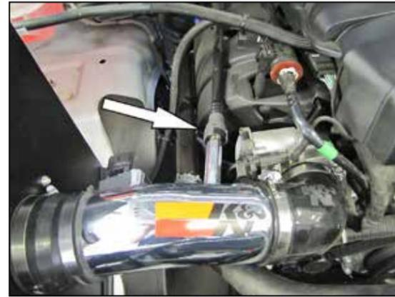
20. Connect the crank case vent hose to the fitting installed into the K&N® intake tube.
