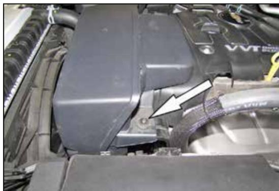
3. Remove the bolt that secures the intake plenum to the engine.
