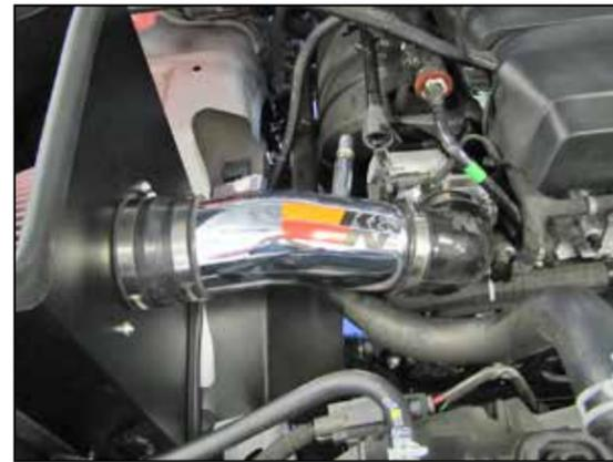
19. Install the Intake tube assembly into the coupling hose at the filter adapter and then connect it to the throttle body, adjust the tube, hoses and heat shield for best fit and then secure with the provided hose clamps and hardware.
