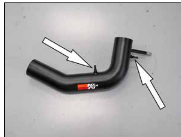
18. Install the two provided NPT vent fittings into the K&N® intake tube as shown. NOTE: On vehicles that only have one vent line, install the provided 1/4npt plug in its place. NOTE: Plastic NPT fittings are easy to cross thread. Install the vent fitting "hand" tight, then turn it two complete turns with a wrench.
