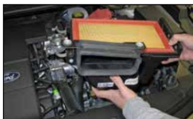
7. Remove the lower air box/fresh air duct from the vehicle.
