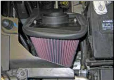
13. Flex the heat shield in on the rubber mounted studs for clearance to install the K&N® air filter. Install the air filter and secure it with the provided hose clamp.
