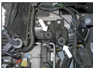
8. Remove the two air box mounting grommets shown.
