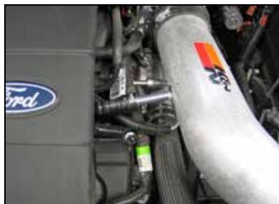
22. Connect the crank case vent hose to the K&N® intake tube.
