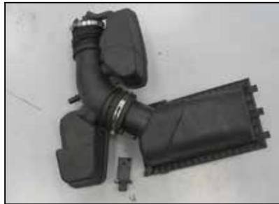
18. Remove the two screws securing the mass air sensor, then remove mass air sensor from the factory air box.
