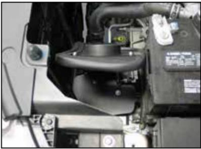
12. Install the heat shield assembly onto the rubber mounted studs and secure with the provided hardware.
