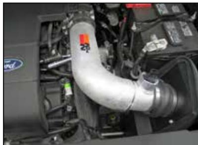
21. Install the K&N® intake tube into the silicone hose at the throttle body and then into the silicone hose on the filter adapter; secure with the provided hose clamp.
