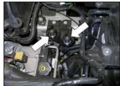
9. Install the two provided rubber mounted studs onto the air box mounting bracket as shown.
