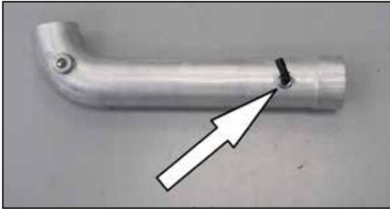
25. Install the 90°, 1/2" vent fitting into the K&N® intake tube as shown.
