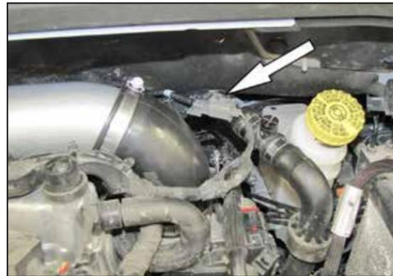
18. Connect the inlet air temperature extension harness to the factory harness.
