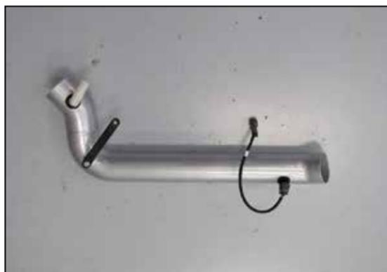
16. Connect the inlet air temperature extension harness provided to the sensor as shown.
