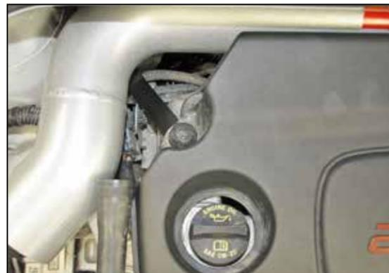
19. Install the engine cover and align the tube mounting bracket then secure the bracket and engine cover using the factory bolt from step #2.
