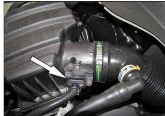
5. On vehicles equipped with a mass air sensor, Disconnect the wiring harness from the sensor.
