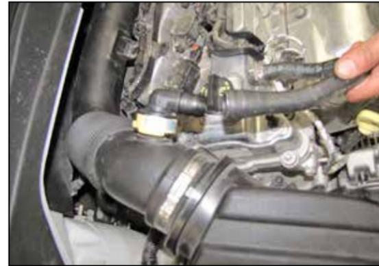
6. Disconnect the crank case vent hose from the fitting in the intake tube.
