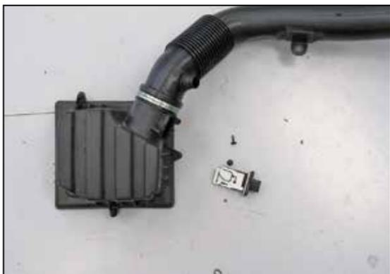
9. On vehicles equipped with a mass air sensor, remove the two screws securing the sensor into the factory air filter housing and then remove the sensor as shown.
