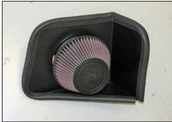
27. Install the K&N® air filter onto the filter adapter and secure with the provided hose clamp.
