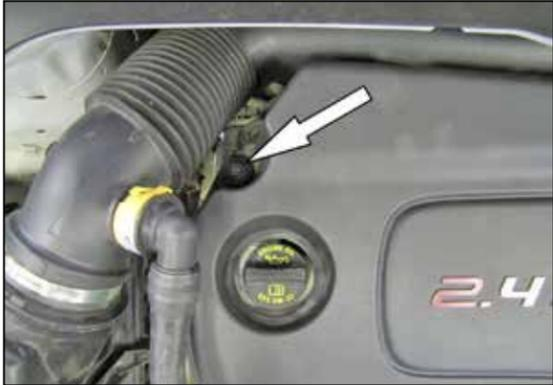
2. Remove the bolt securing the engine cover and then remove the engine cover from the vehicle.
