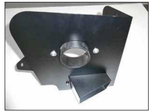
6. Install the K&N® air filter adapter and fresh air inlet duct into the heat shield and secure with the provided hardware.
