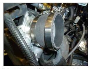
11. Install the provided straight coupler onto the throttle body and secure with the provided hose clamp.
