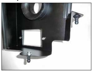
8. Install the two provided mounting studs onto the heat shield as shown and secure with the provided hardware.
