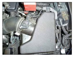
2. Unplug the mass air sensor electrical connection.
