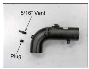
22. On vehicles not equipped with an EVAP hose connected to the intake tube, install the provided NPT plug onto the K&N® intake tube. On vehicles Equipped with an EVAP hose to the Intake tube, install the 5/16" vent fitting into the K&N® intake tube.
