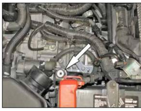
16. Install the 1" rubber mounted stud onto the front air box mounting location as shown.
