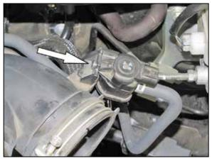
8. Unbolt the EVAP solenoid from the mounting bracket.
