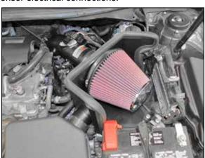
29. Install the K&N® air filter onto the filter adapter and secure with the provided hose clamp. NOTE: Drycharger® air filter wrap; part # RF-1048DK is available to purchase separately. To learn more about Drycharger® filter wraps or look up color availability please visit http://www.knfilters.com®.
