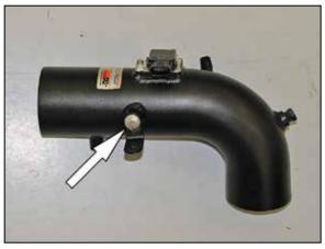
23. Install the EVAP bracket (070066) onto the K&N® intake tube using the provided hardware. NOTE: Do not completely tighten the bracket at this time.
