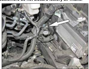
10. Remove the bolt securing the rear air box mounting bracket to the strut tower and then remove the bracket from the strut tower.
