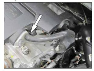
27. Install the provided silicone hose onto the vent fitting installed into the K&N® intake tube and then to the fitting on the valve cover as shown. NOTE: Some trimming of the vent hose may be necessary for proper fit.
