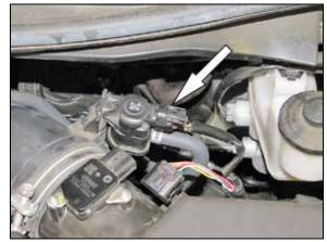
3. Disconnect the EVAP solenoid electrical connection.
