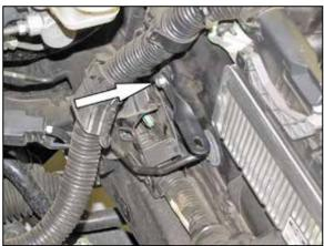
15. Install the heat shield mounting bracket (070702) onto the inner fender air box mounting location from step #10.
