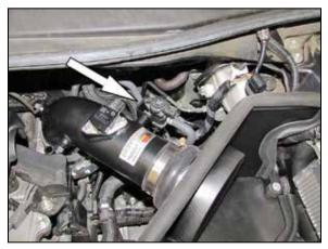
26. Secure the EVAP solenoid to the bracket installed onto the K&N® intake tube during step #23 using the provided hardware. Adjust the solenoid and bracket for best fit and then tighten the bolt securing the bracket.
