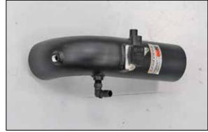
21. Install the 90° vent fitting into the K&N $^{\! 8}$  intake tube as shown.
