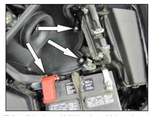
17. Install the heat shield into the vehicle so the fresh air duct slides over the tube on the heat shield and the heat shield sits on the mounting locations. Secure the heat shield to the rubber mounted studs and brackets with the provided hardware.
