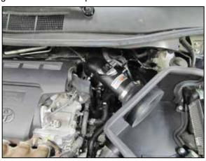
25. Install the K&N® intake tube assembly into the silicone hose at the throttle body, align with the filter adapter and then slide the hump hose onto the filter adapter. Secure the hose with the provided hose clamps.
