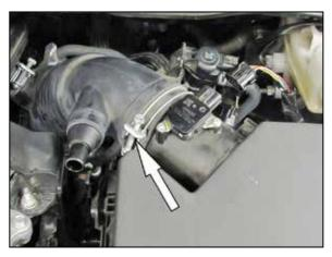
5. Loosen the hose clamp securing the intake hose to the air box lid.
