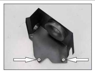
12. Install the two ½" rubber mounted studs onto the heat shield as shown.
