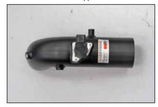
20. Install the mass air sensor into the K&N $^{\circ}$  intake tube and secure with the provided hardware.
