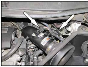
28. Reconnect the EVAP solenoid and Mass air sensor electrical connections.
