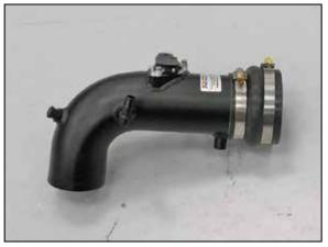
24. Install the provided hump hose (084079) all the way onto the K&N® intake tube as shown. Do not tighten the hose clamps at this time.
