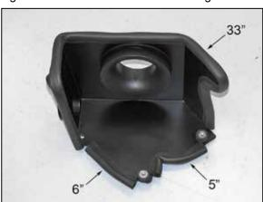
14. Install the edge trim onto the heat shield as shown.
