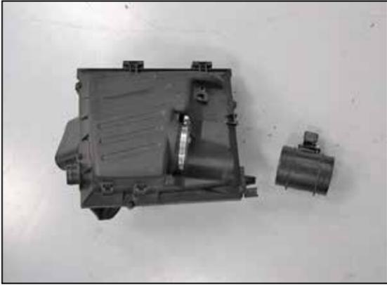
7. Loosen the hose clamp that secures the mass air sensor housing to the air box then remove mass air sensor housing from air box.
