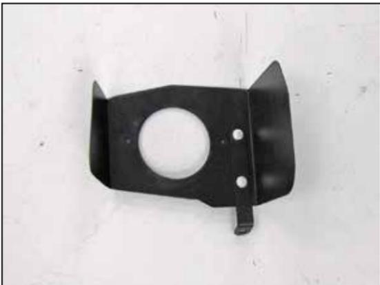
9. Install heat shield bracket (064322) to heat shield as shown.
