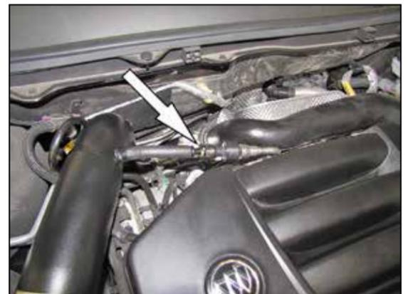
21. Reconnect crankcase vent line as shown.
