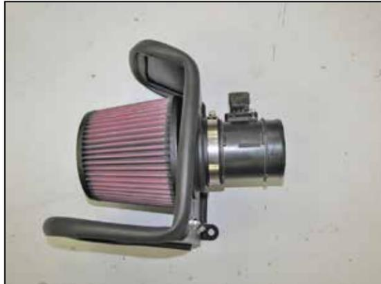
13. Install mass air sensor and housing into filter as shown and secure with the provided hose clamp. **NOTE: The arrow on the mass air housing indicating air flow should point away from filter.**
