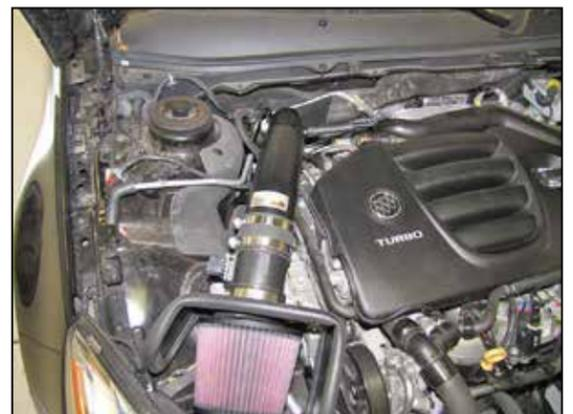
20. Install the intake tube assembly into the hose on turbo then into hose on mass air housing. Align intake tube with heat shield assembly. Secure with provided hose clamps as shown.
