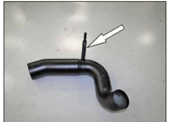
19. Install hose assembly onto intake tube as shown.
