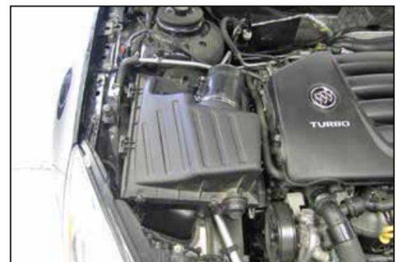
6. Lift up the air box to dislodge it from the mounting grommets; then remove from vehicle.
