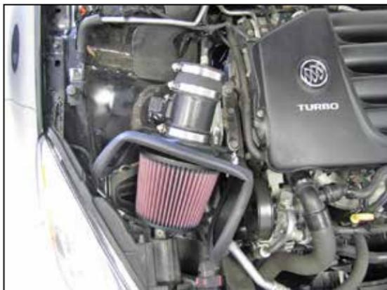
16. Install heat shield assembly and secure it to the motor mount bolt removed in step 15 as shown.
