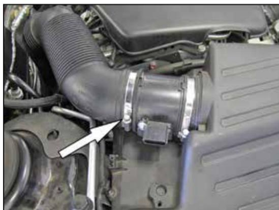
4. Loosen the hose clamp that secures the intake tube to the mass air sensor housing.
