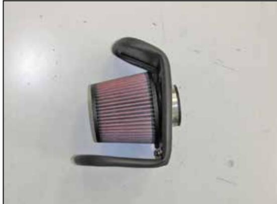
12. Insert filter through heat shield opening as shown.
