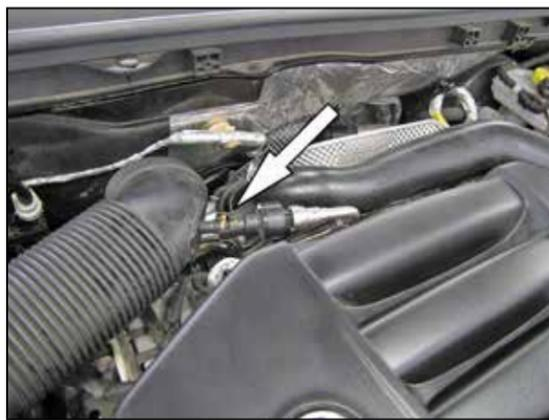
3. Release locking clip and remove crank case vent line from intake tube.
