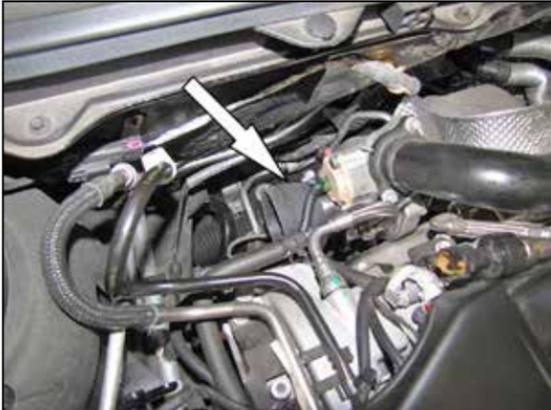
8. Install hose (084016) onto turbo inlet. Secure with provided hose clamp.
