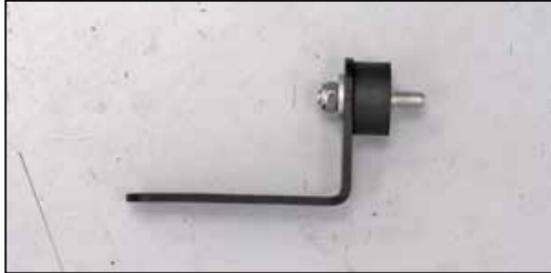
15. Install the rubber mounted stud onto the mounting bracket (010031) and secure with the provided hardware.
