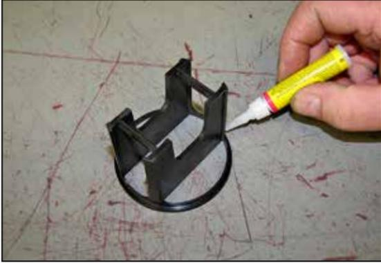
11. Apply several drops of the provided "Super Glue" onto the air guide as shown.
