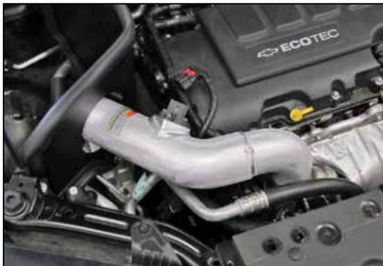
17. Install the tube assembly into the silicone hose on the turbo inlet and align so the rubber mounted stud protrudes through the heat shield. Secure the tube with hose clamp and hardware provided.
