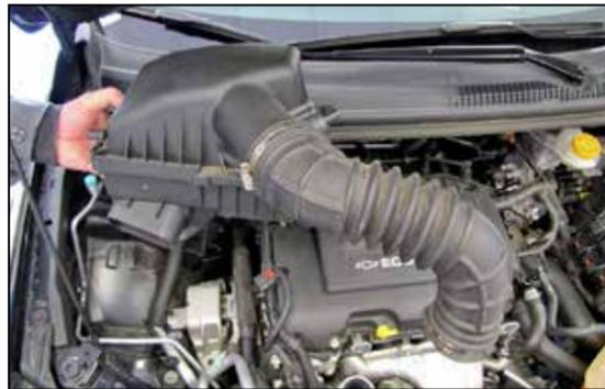
4. Disconnect the intake tube from turbo inlet, and then lift up the air box to dislodge it from the mounting grommets and then remove the air box assembly from the vehicle.
