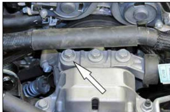
5. Remove the rear engine mount bolt shown. **NOTE: This bolt will be reused.**
