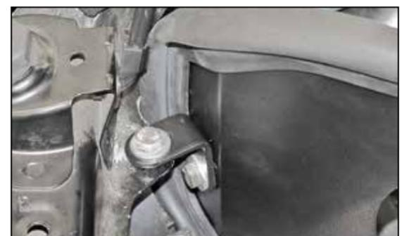
9. Install the provided "L" bracket (070066) onto the core support and heat shield as shown using the provided hardware, then tighten all of the heat shield mounting hardware. **NOTE: The slotted end of the bracket will attach to the core support.**
