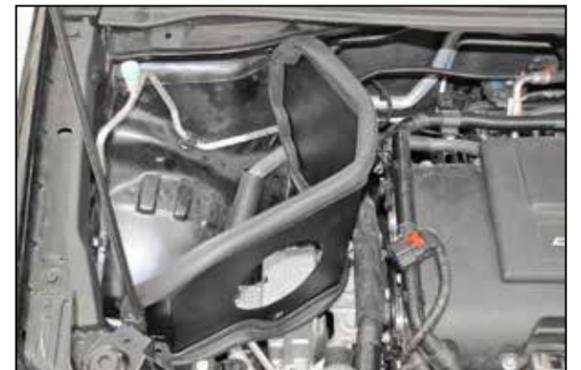
8. Install the heat shield assembly onto the engine mount and secure with the bolt removed in step #5. **NOTE: Do not completely tighten at this time.**
