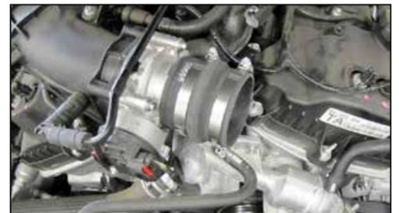
9. Install the provided silicone hose (08696) onto the throttle body and secure with the provided hose clamp as shown.
