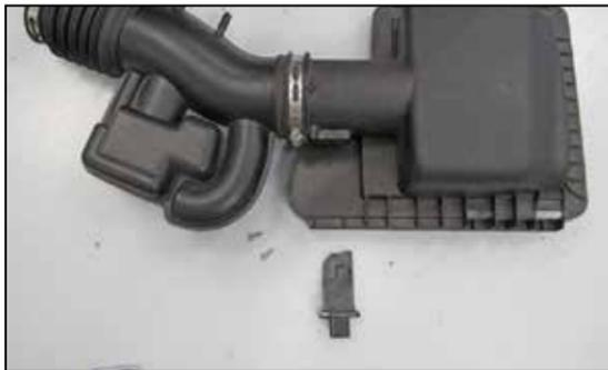
17. Remove the two screws securing the mass air sensor into the factory air box and then remove the mass air sensor.
