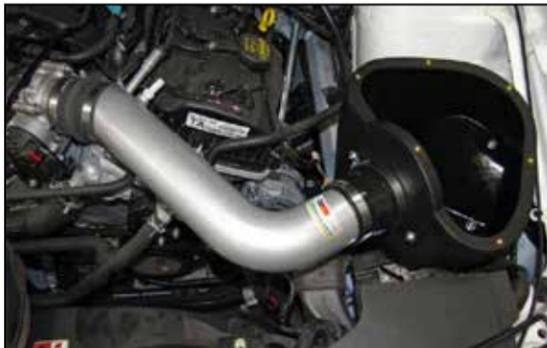
19. Install the K&N® intake tube into the silicone hose at the throttle body and then into the silicone hose on the filter adapter, secure the intake tube with the provided hose clamps.
