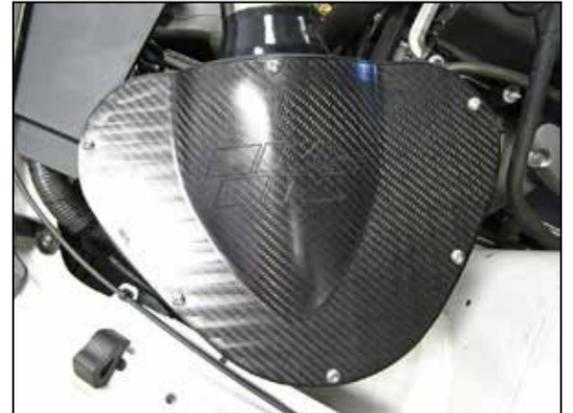
22. Install the air box cover and secure with the provided hardware.
