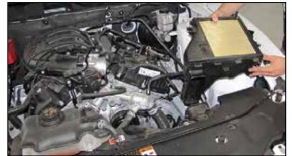
8. Remove the lower air box housing from the vehicle.
