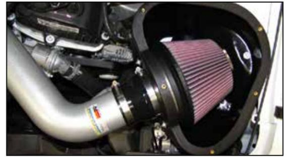
21. Install the K&N® air filter onto the filter adapter and secure with the provided hose clamp.
