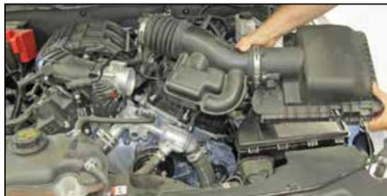
6. Remove the upper air box/tube assembly from the vehicle.
