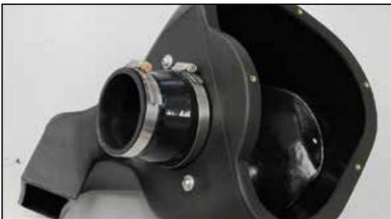
12. Install the provided silicone hose (08724) onto the K&N® filter adapter and secure with the provided hose clamp.
