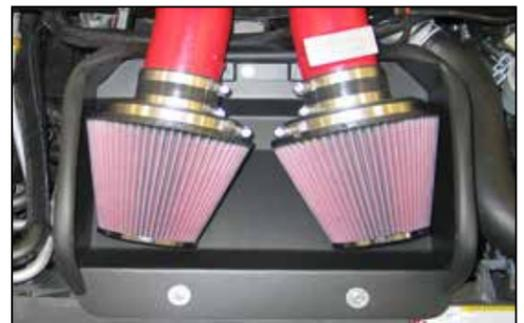
22. Install the filter assemblies onto the intake tubes and secure with the provided hose clamps.
