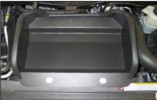
10. Install the heat shield onto the air box mounting location and secure with the provided hardware.
