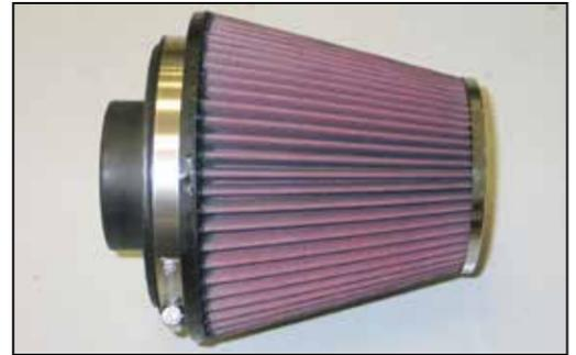
20. Install the filter adapters into the K&N® air filters and secure with the provided hose clamps.
