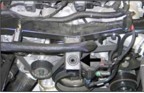
7. Remove the rubber mounting grommet shown.
