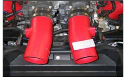
19. Align the intake tubes so that they are straight and even coming out of the throttle bodies, then tighten the heat shield mounting bolts and tube mounting bolts.
