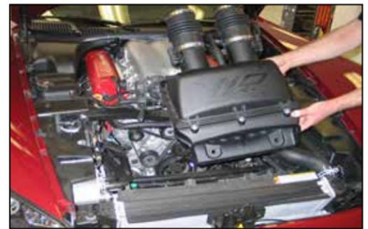
6. Dislodge the air box assembly from the mounting grommet and remove the air box from the vehicle. **NOTE: K&N Engineering, Inc., recommends that customers do not discard factory air intake.**
