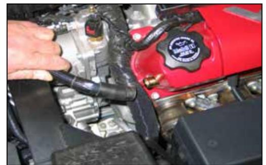
5. Cut the tie wrap which secures the vent hose to the valve cover port. Then unhook the crank case vent hose as shown.
