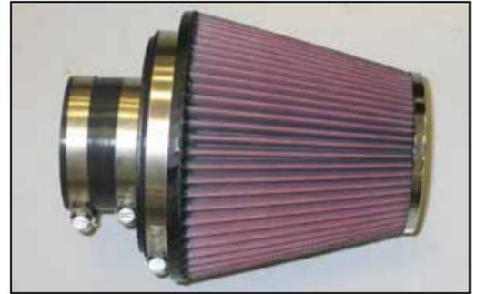
21. Install the silicone hoses (08698) onto the filter adapters and secure with the provided hose clamps.
