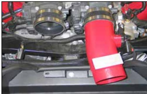
17. Install the left side K&N® intake tube into the silicone hose at the throttle body while connecting the crank vent line to the vent fitting. Secure the tube to the bracket with the provided hardware.
