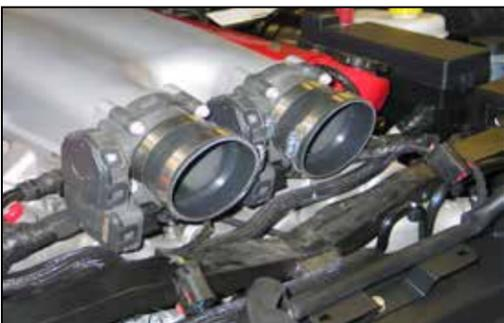
12. Install the silicone hoses (084091) onto the throttle bodies and secure with the provided hose clamps.
