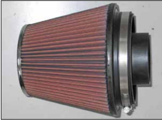
22. Install the provided air filter adapter into the K&N® air filter and secure with the provided hose clamp.
