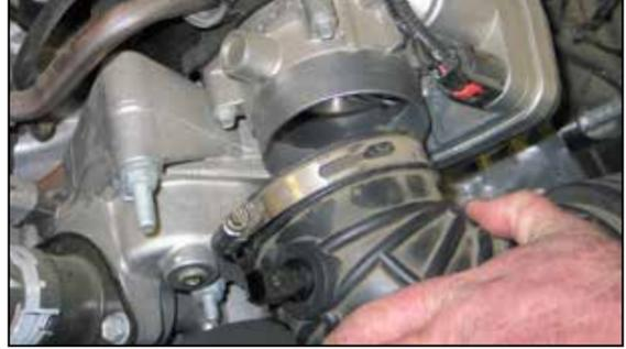
4. Loosen the hose clamp that secures the intake tube to the throttle body and pull the intake tube off of the throttle body.
