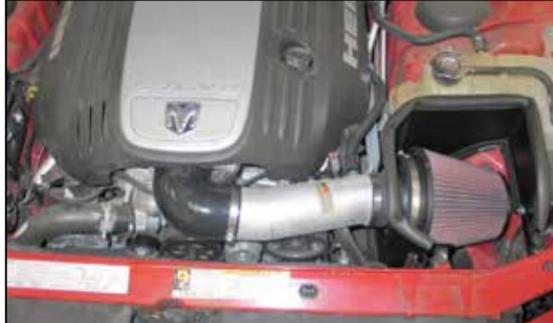
25. Reinstall the engine cover onto the engine.
