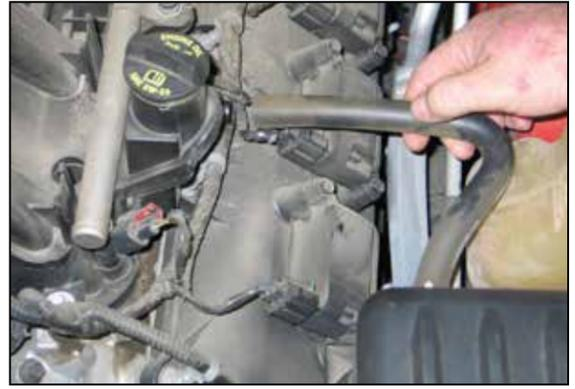
5. Disconnect the crankcase vent hose from the valve cover port as shown.
