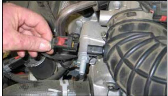
3. Release the red locking tap and then disconnect the inlet air temperature sensor electrical connection.
