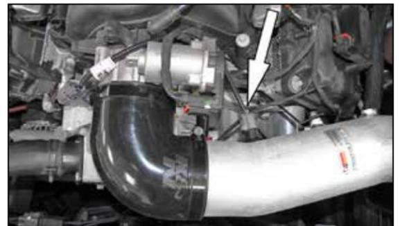
21. Connect the provided inlet air temperature sensor harness extension into the factory harness, run it under the throttle body and then connect to the inlet air temperature sensor as shown. Using the provided cable tie, secure the harness extension tube mounting bracket.
