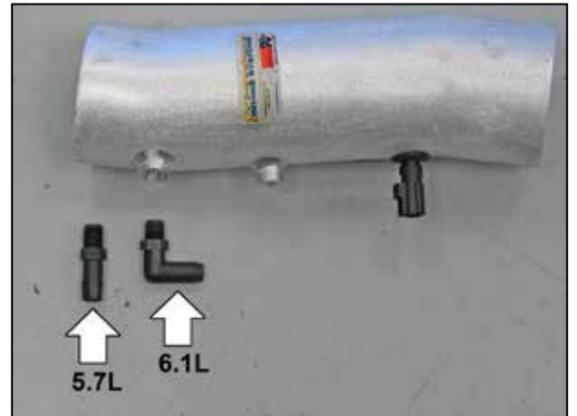
18. Install the appropriate 1/4npt fitting into the K&N® intake tube. The 90° fitting is for 6.1L engine size and the straight fitting is for 5.7L engine size.
