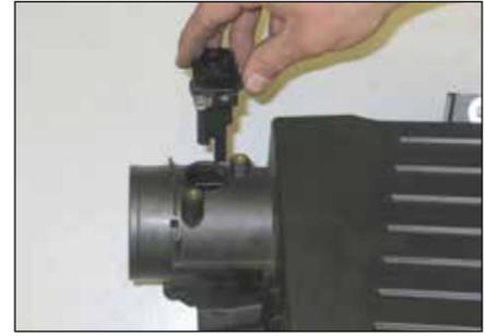
21. Remove the mass air sensor from the stock air box.
