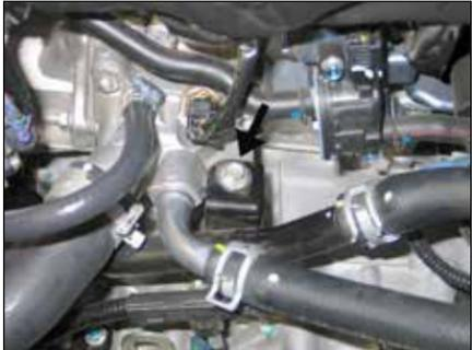
12. Remove the bolt shown that secures the heater hose mounting bracket to thermostat housing.
