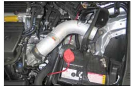
23. Install the K&N intake tube into the silicone hose at the throttle body and align with the tube mounting bracket installed in step #13. Secure with the provided hose clamp and hardware.
