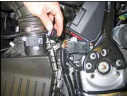
2. Disconnect the mass air sensor electrical connection and then unhook the wiring harness from air box.
