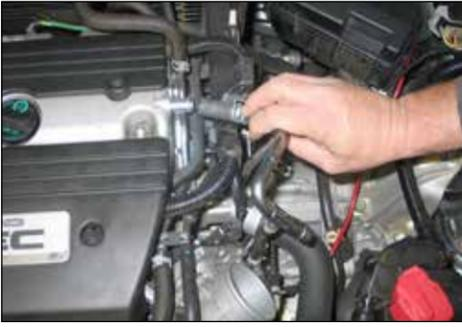
9. Release the spring clamp which secures the crank case vent hose to the valve cover and then unhook crank case vent hose from the valve cover as shown.
