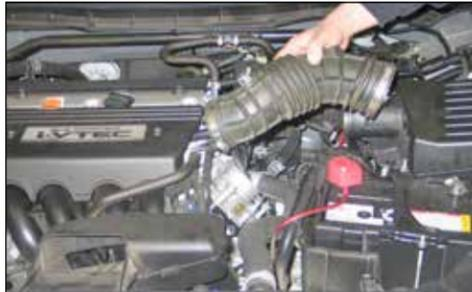
5. Remove the stock intake tube from the vehicle.
