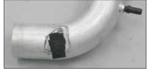
22. Install the mass air sensor into the K&N intake tube and secure with the provided hardware.
