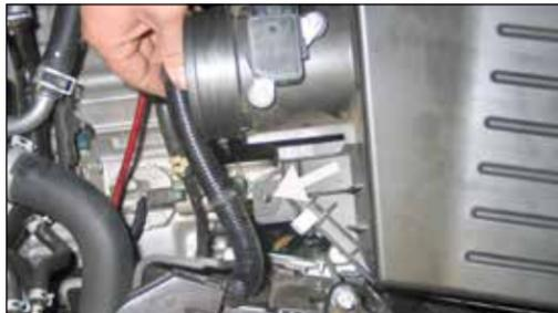
6. Unhook the wiring harness from the air box as shown.
