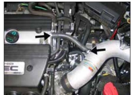
24. Install the provided crankcase vent hose onto the valve cover port and then to the vent fitting on the K&N intake tube.
