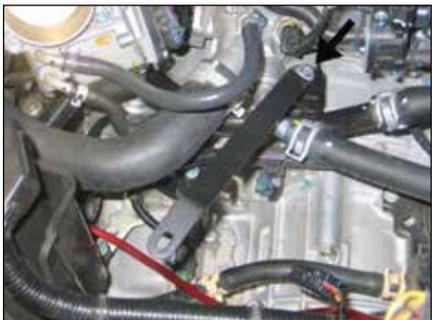
13. Using the provided bolt, secure the intake tube mounting bracket (070124) to the heater hose mounting bracket and thermostat housing from step #12.
