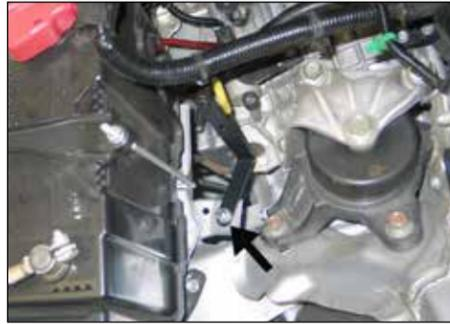
16. Install the front heat shield bracket (070123) onto the lower front air box mounting location using the provided hardware.
