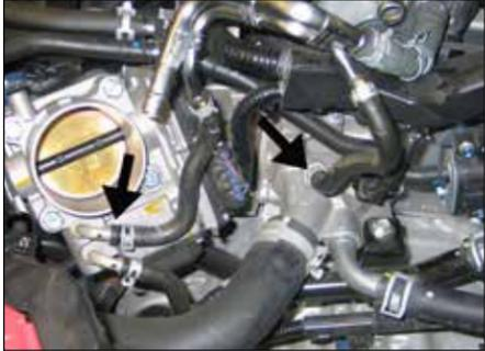
10. Release the two spring clamps securing the coolant bypass hoses to the throttle body and thermostat housing, then remove the bypass hose assembly from the vehicle.
