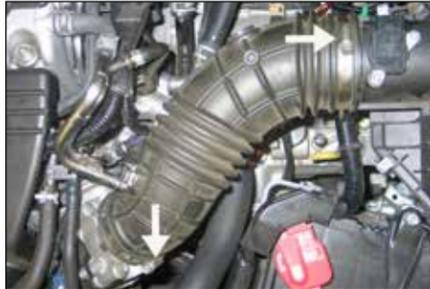
4. Release the two hose clamps securing the intake tube to the air box and throttle body.
