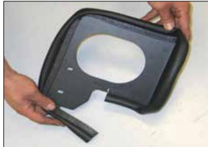
17. Install the edge trim onto the heat shield as shown.
