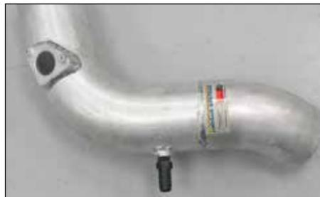
20. Install the provided vent fitting into the K&N intake tube as shown.
