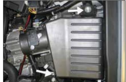
7. Loosen and remove the two air box mounting bolts.
