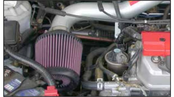
22. Install the K&N air filter onto the K&N intake tube and secure with the provided hose clamp. Adjust for best fit and clearance then tighten all hardware.
