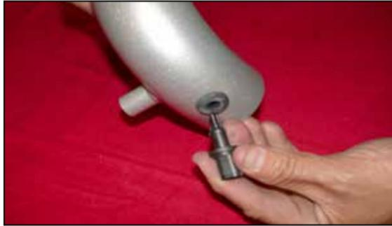
17. Install the provided rubber grommet into the hole on the K&N intake tube, then install the air temperature sensor into the grommet as shown.
