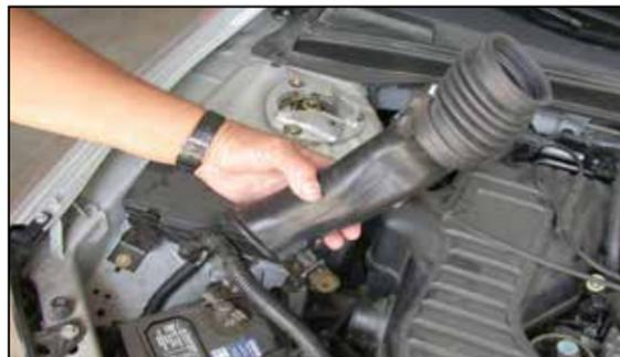
5. Remove the air inlet duct.
