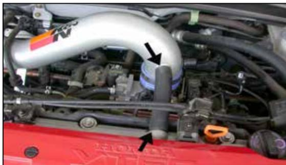
20. Install the provided silicone hose onto the crankcase vent on the cam cover, then connect the other end to the vent on the K&N intake tube as shown.
