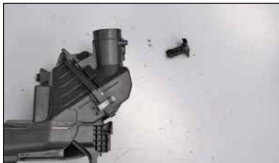
16. Remove the mass air sensor from the factory air filter housing.
