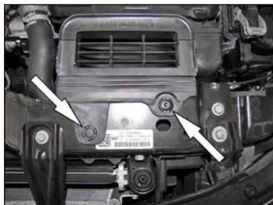
4. Remove the two plastic clips that secure the intake air diverter and then lift off the air diverter.
