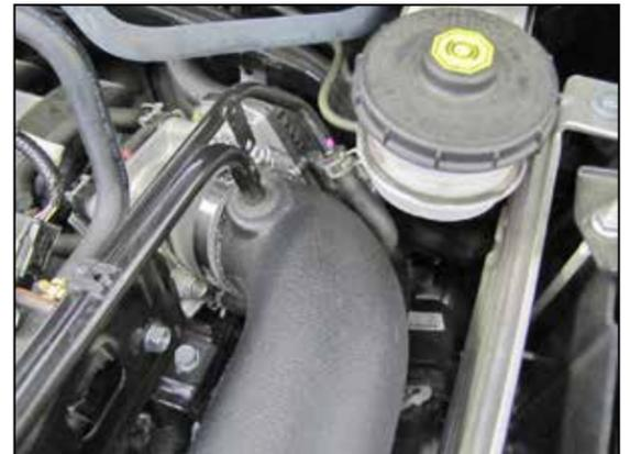
20. Install the crank case vent tube into the grommet installed into the K&N intake tube.
