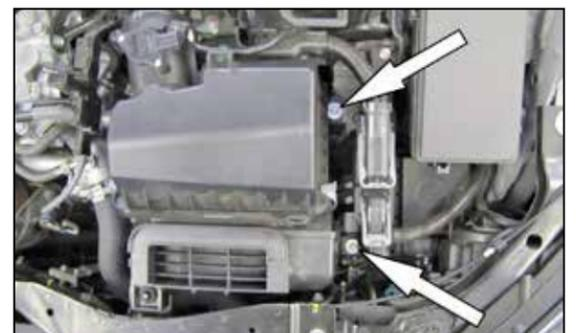
6. Loosen the two bolts that secure the air filter housing, apply some spray lubricant to the mounting grommet and then remove the air filter housing from the vehicle.
