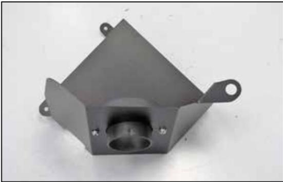
8. Install the filter adapter into the heat shield as shown and secure with the provided hardware.
