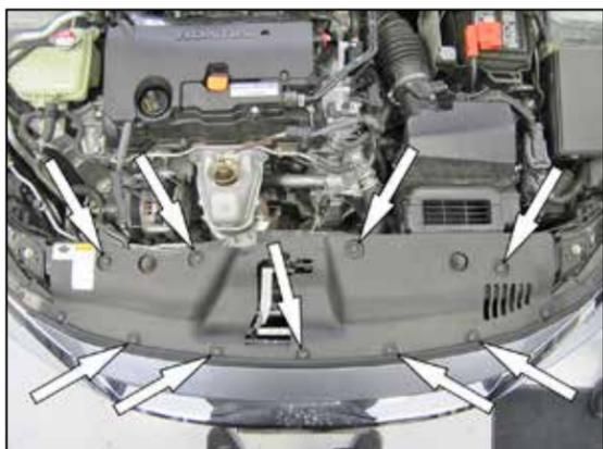
2. Remove the nine clips that secure the core support cover and then remove the cover from the vehicle.
