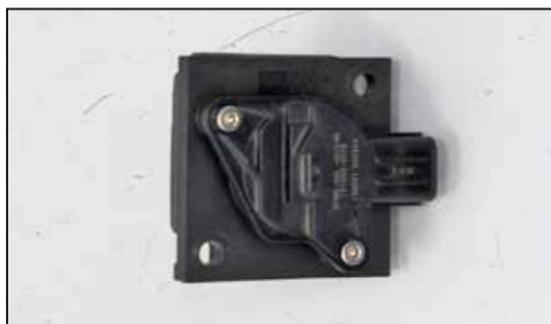
17. Install the mass air sensor into the K&N mass air adapter and secure with the provided hardware.
