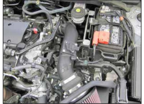
19. Install the K&N intake tube into the coupling hoses, adjust for best fit and then secure with the provided hose clamps.
