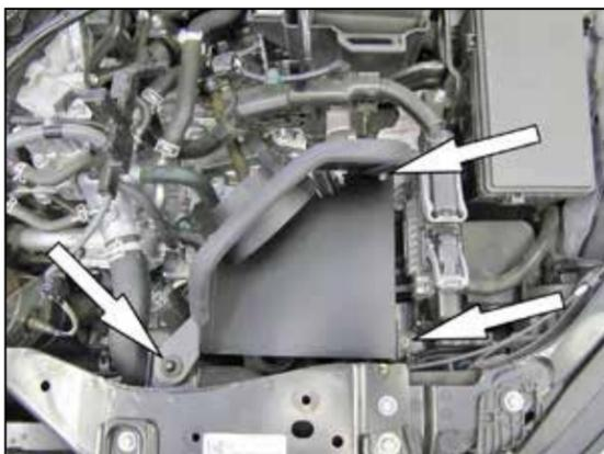
11. Install the heat shield assembly into the vehicle and secure with the provided hardware and factory grommet.
