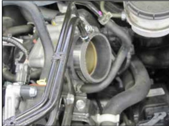
14. Install the coupling hose (08284) onto the throttle body and secure with the provided hose clamp.
