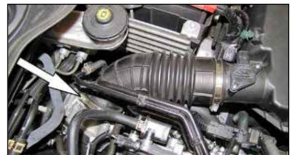
5. Loosen the two hose clamps that secure the intake tube to the air filter housing and the throttle body, Loosen the spring clamp securing the crank case vent hose and then remove the intake hose from the vehicle.
