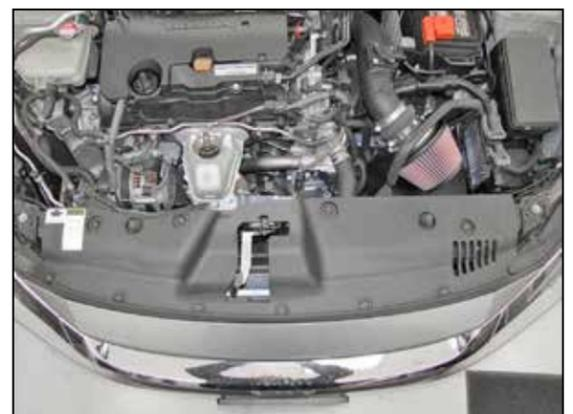
22. Reinstall the core support cover and secure with the factory retaining clips.
