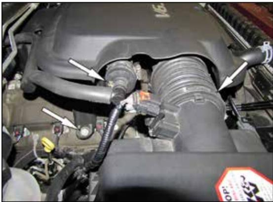
2. Loosen the hose clamp that secures the intake hose to the air filter housing. Using a screwdriver, unlock the small clamp that secures the vent line to the connector and then disconnect the vent line. Remove the bolt securing the intake plenum to the engine.
