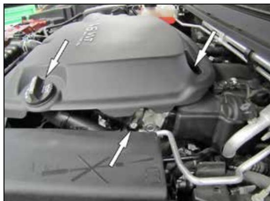
3. Remove the oil fill cap and loosen the hose clamp securing the intake hose to the throttle body. Remove the bolt securing the intake plenum to the engine.
