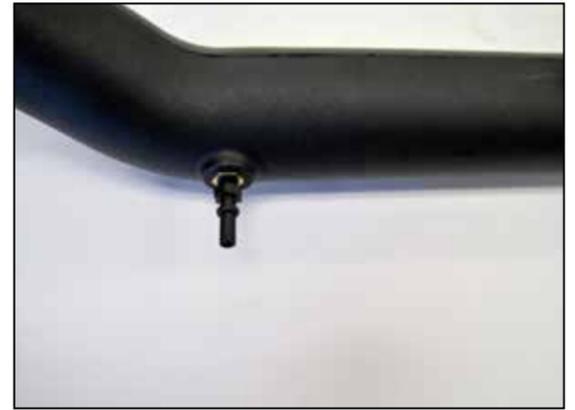
17. Install the quick connect fitting into the K&N® intake tube as shown.
