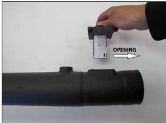
14. Install the mass air sensor assembly into the K&N® intake tube as shown, secure the sensor with the provided hardware.
