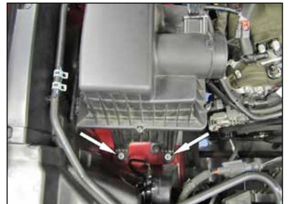
6. Remove the two nuts securing the air filter housing to the inner fender and then remove the housing from the vehicle.
