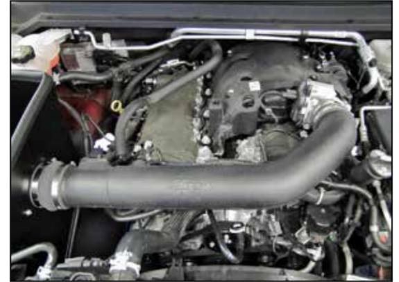
18. Install the provided hump coupler (08699) onto the K&N® intake tube, then install the intake tube assembly into the coupler at the throttle body and align with the filter adapter. Slide the hump coupler onto the filter adapter, adjust the tube for best fit and secure with the provided hose clamps.
