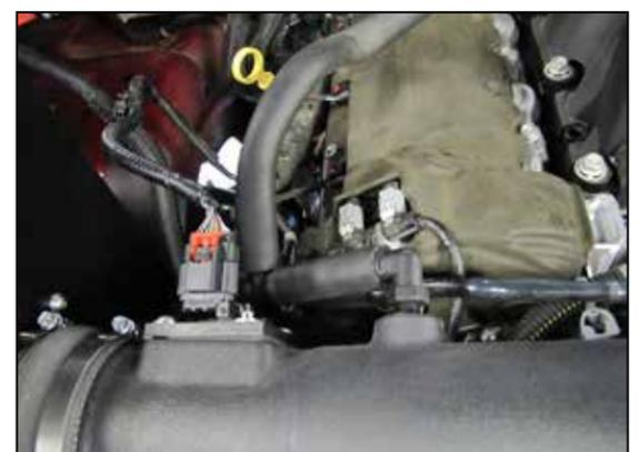
20. Using the provided vent hose, connect the factory vent to the 90° fitting installed into the K&N® intake tube. Reconnect the mass air sensor electrical connection.
