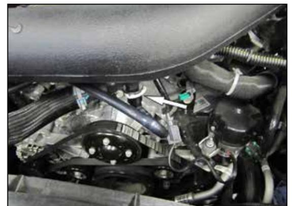
19. Rotate the crank case vent line and fitting so it aligns with the quick connect fitting and then connect.
