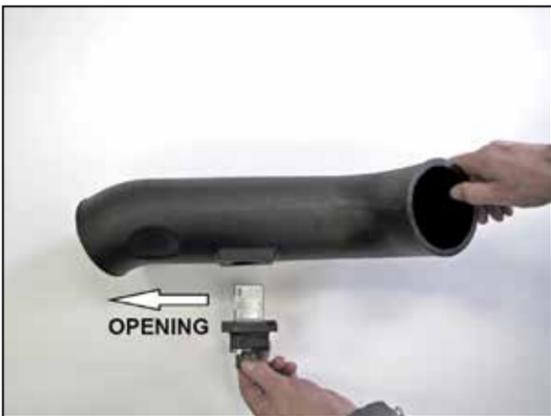
11. Install the sensor assembly into the K&N® intake tube and secure with the provided hardware. **NOTE: Be sure to install the sensor in the correct direction, the opening in the sensor should be pointed towards the filter end of the tube.**
