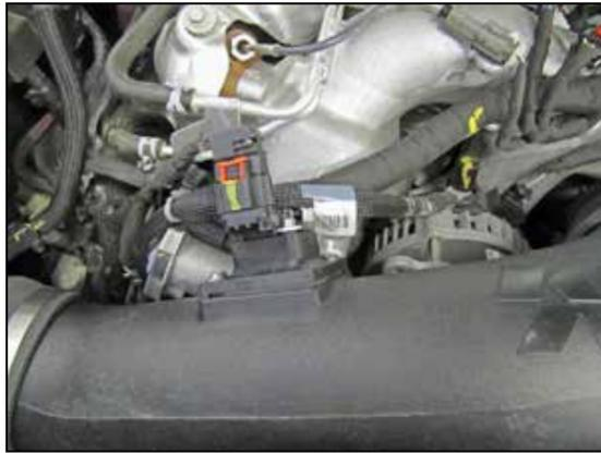
13. Reconnect the mass air sensor electrical connection and secure the red locking tab.
