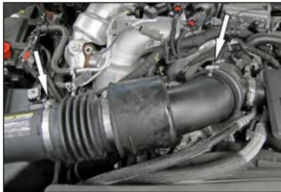
3. Loosen the two hose clamps securing the factory intake tube to the turbo inlet and air filter housing, then remove the factory intake tube from the vehicle.
