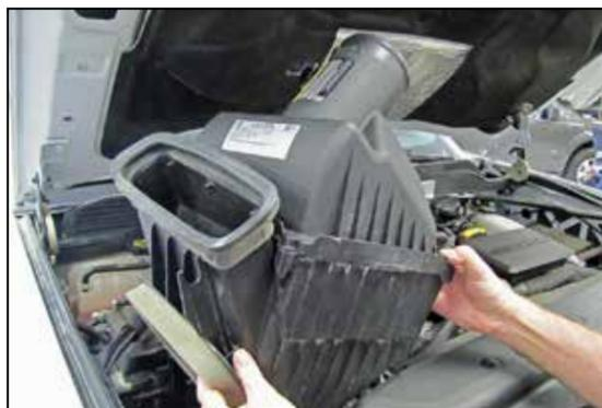
4. Lift up the air filter housing to release it from the mounting grommets and then remove the air filter housing from the vehicle.
