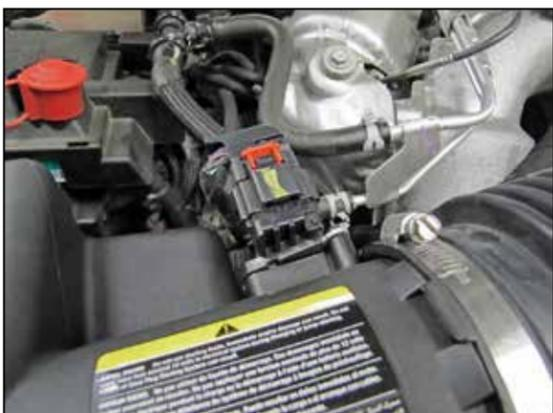
2. Slide the red locking tab back and then release the mass air sensor electrical connection.
