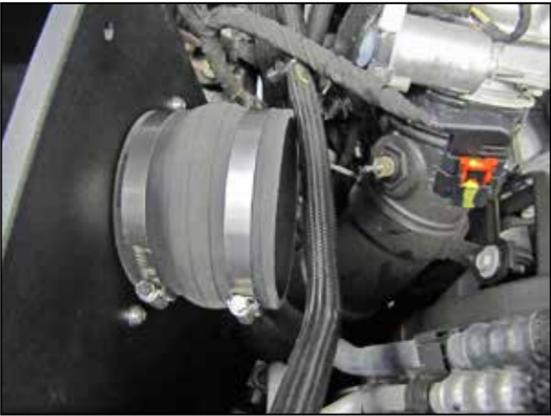
8. Install the provided hump coupler (08418) onto the filter adapter and secure with the provided hose clamp.
