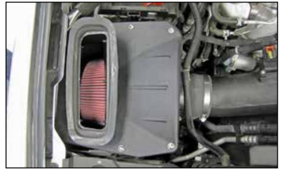
17. Install the K&N® air filter housing lid onto the filter housing and secure with the provided hardware.
