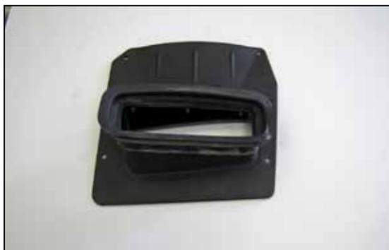
16. Install the bellows onto the K&N® air filter housing lid and secure with the factory retaining clips.
