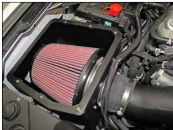
14. Install the K&N® air filter into the air filter housing and then onto the filter adapter. Secure the filter with the provided hose clamp.
