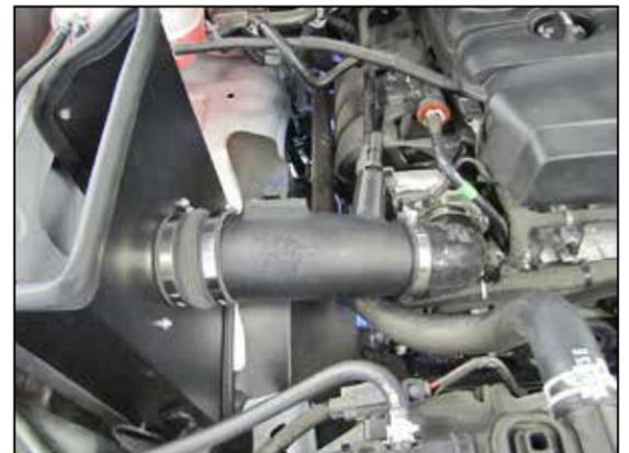
21. Install the Intake tube assembly into the coupling hose at the filter adapter and then connect it to the throttle body, adjust the tube and hoses for best fit and then secure with the provided hose clamps.
