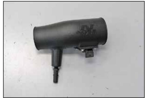
18. Install the Provided NPT quick disconnect fitting into the K&N intake tube as shown.
