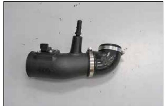
20. Install the provided angled coupling hose (084087) onto the intake tube as shown.
