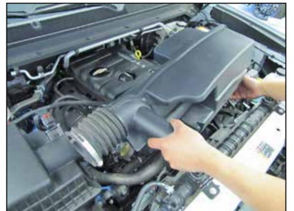
5. Remove the intake plenum from the vehicle.
