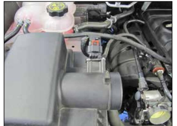
6. Disconnect the mass air sensor electrical connection.
