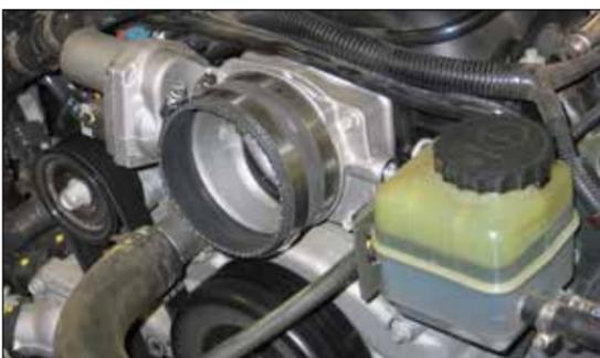
14. Install the silicone hose (08618) onto the throttle body and secure with the provided hose clamp.
