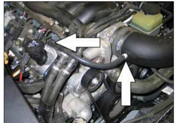
23. Connect the crank case vent hose to the valve cover port and then connect the open end to the vent fitting installed into the K&N intake tube.
