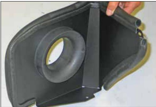
12. Install the filter adapter into the heat shield and secure with the provided hardware.
