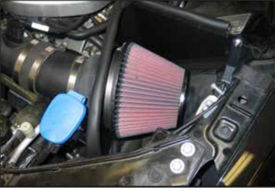
25. Install the air filter and secure with the provided hose clamp.
