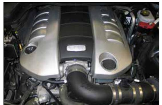
24. Remove the oil fill cap and reinstall the engine cover. Reinstall the oil fill cap.
