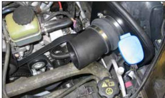
18. Install the small intake tube into the silicone hose at the filter adapter as shown.
