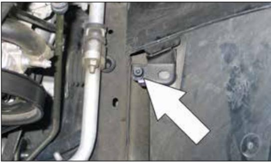
9. Remove the air box mounting stud shown.
