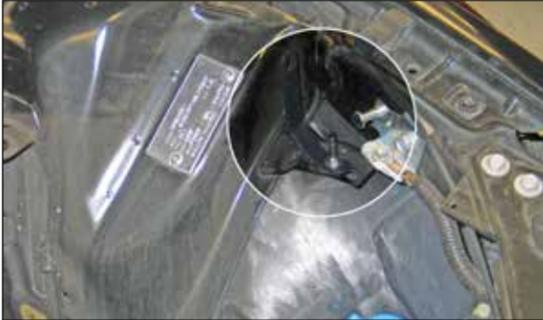
10. Install the heat shield mounting bracket (07190) onto the air box mounting stud using the provided hardware.
