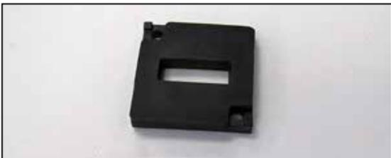
10. Install the provided gasket onto the K&N® mass air sensor adapter.
