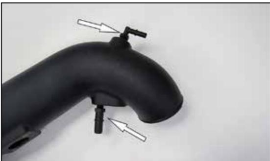
9. Install the provided fittings into the K&N® intake tube as shown.
