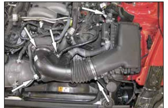
5. Disconnect the EVAP vent line, cut the clamp for the sound tube at the sound drum and disconnect the hose from the drum. Loosen the hose clamps that secure the intake tube to the throttle body and air filter housing then remove the intake tube from the vehicle.
