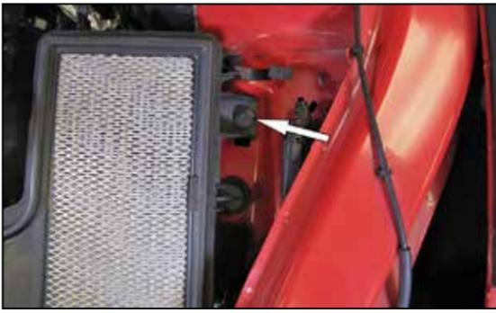
7. Remove the bolt that secures the air filter housing to the inner fender and then remove the lower air filter housing from the vehicle.
