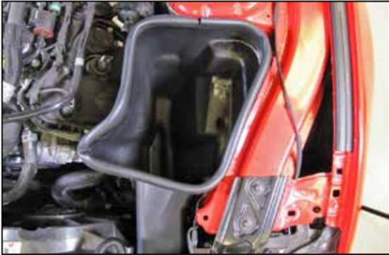
8. Install the provided edge trim onto the K&N® air filter housing. Install the K&N® air filter housing into the vehicle and secure with the provided hardware. **NOTE: Some trimming of the edge trim will be necessary.**
