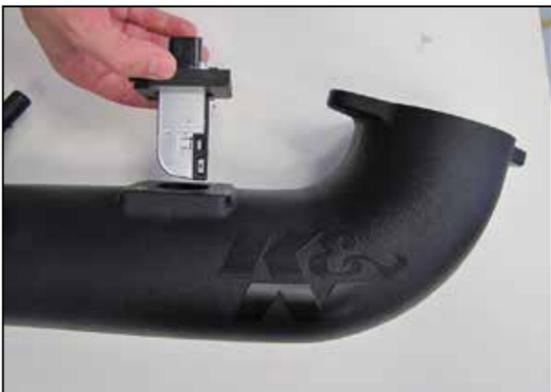
12. Install the mass air sensor assembly into the K&N® intake tube as shown and secure with the provided hardware.
