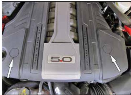
3. Remove the fastener covers on the engine cover, remove the two nuts that secure the cover and then remove the cover from the engine.
