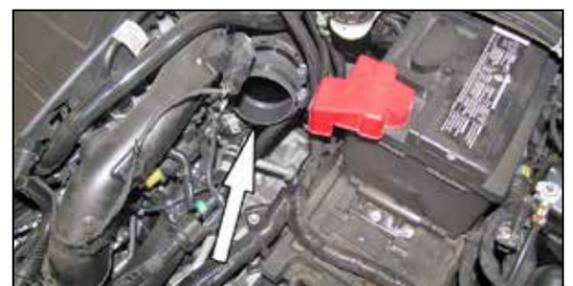
8. Install the provided hump hose (087121) onto the turbo inlet and secure with the provided hose clamp.
