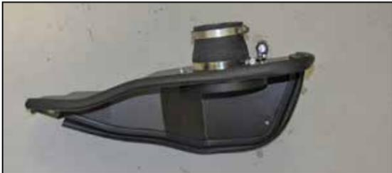
13. Install the provided step coupler (084055) onto the filter adapter and secure with the provided hose clamp.
