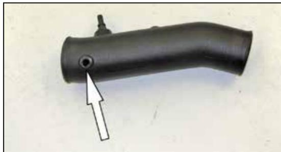
18. Install the provided inlet air temperature sensor grommet into the K&N® intake tube.
