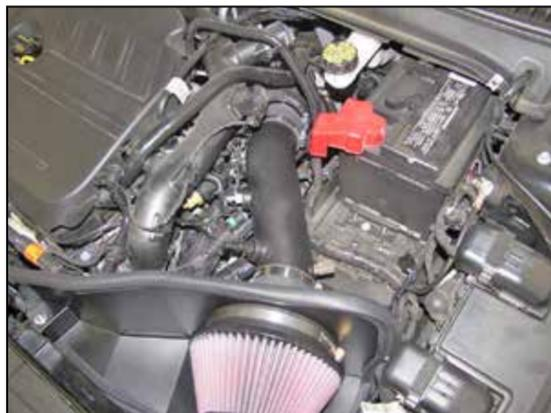
21. Install the K&N® intake tube assembly into the coupling hose at the turbo inlet and then into the coupling hose at the filter adapter. Adjust the tube for best fit and then secure with the provided clamps.
