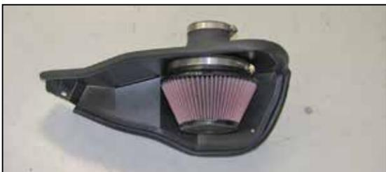
14. Install the K&N® air filter onto the filter adapter and secure with the provided hose clamp.
