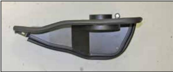
12. Install the filter adapter into the heat shield and secure with the provided hardware.
