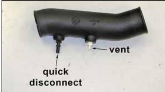
17. Install the provided 1/4" npt fittings into the K&N® intake tube as shown.
