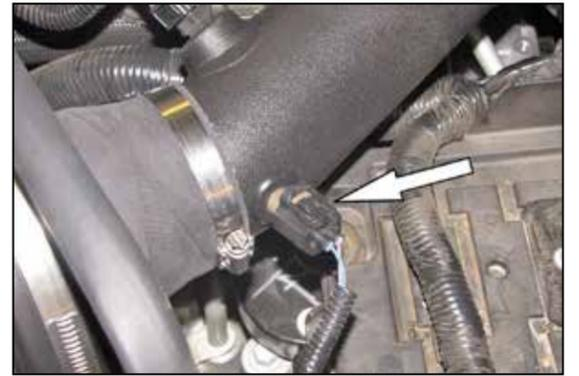
23. Connect the inlet air temperature sensor electrical connection.
