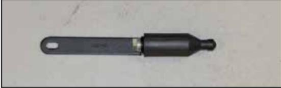
10. Install the heat shield mount onto the provided bracket (064320) as shown.
