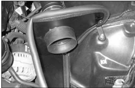
17. Clip the edge trim to the outside of the heat shield (cut any excess trim). Fit the heat shield to the intake pipe assembly; ensure the rubber adapter lip sits up against the shield.
