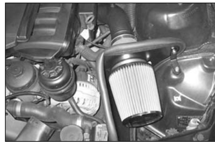
22. Carry out a final check of the alignment / fitment of the K&N induction system, ensuring that all clips etc are tight before starting the engine. Installation is now complete.
