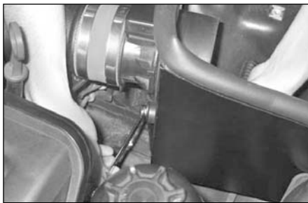
18. Attach the long bracket to the lower mounting hole in the heat shield using a studded mounting, nylock nuts & washers.
