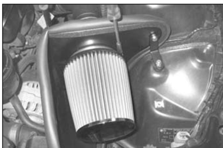
20. Fit the new Filtercharger to the intake pipe / rubber adaptor, ensure the filter sits flush with the heat shield and fully tighten the #64 clip.
