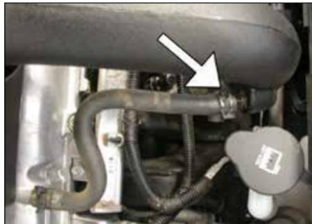
20. Install the stock crankcase vent hose onto the fitting on the K&N® intake tube and secure with the stock hose clamp.
