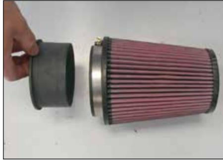
17. Install the filter adapter into the K&N® air filter as shown.
