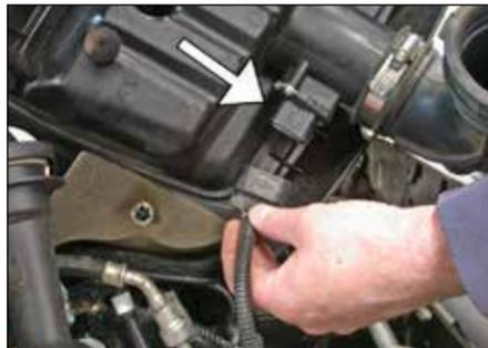
5. Flip the airbox assembly up towards the driver's side of the vehicle to gain access to the mass air sensor electrical connection, and then disconnect the mass air sensor electrical connection as shown.
