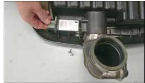
7. Remove the two screws securing the mass air sensor to the stock intake tube and then remove the sensor as shown.
