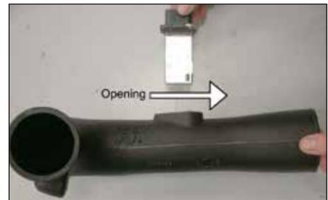
8. Install the mass air sensor into the intake tube as shown.
