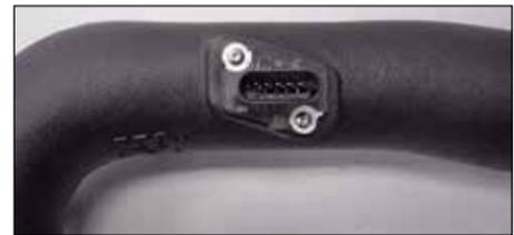
9. Secure the mass air sensor to the intake tube with the screws and spacers provided.
