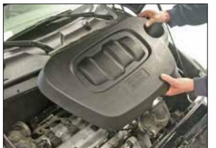
6. Remove the airbox assembly from the vehicle.
