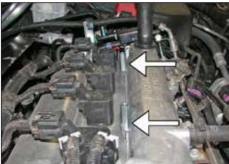
13. Thread and tighten the two coupling nuts onto the studs installed in step #12.
