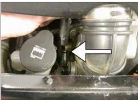
2. Loosen the hose clamp, which secures the crankcase vent hose to the stock intake tube, and then disconnect the crankcase vent hose from the stock intake tube as shown.
