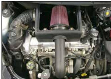
19. Install the K&N® intake tube through the opening in the airbox and into the filter assembly. Then install the intake tube into the silicone hose at the throttle body and secure the filter and tube with the provided hose clamps.
