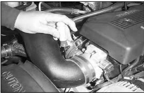
27. Align and check the intake tube for clearance, tighten the hose clamp on the silicone hose at the intake tube.
