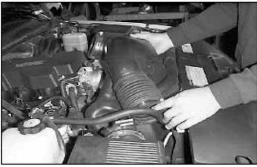
7. Detach the intake tube from the throttle body and remove the intake assembly.
