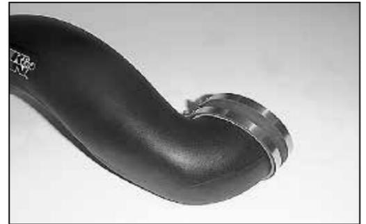
23. Install the 4"ID silicone hose onto the intake tube.
