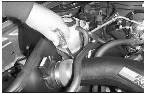
28. Tighten the hose clamp on the silicone hose at the intake tube.
