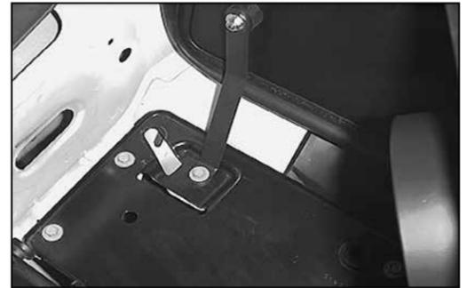
21. Secure the bracket to the airbox mounting tray using the bolt removed in step 19.
