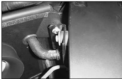
30. Insert the radiator over flow hose into the grommet on the heat shield.
