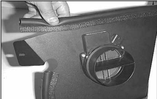
11. Install the trim seal onto the heat shield as shown.
