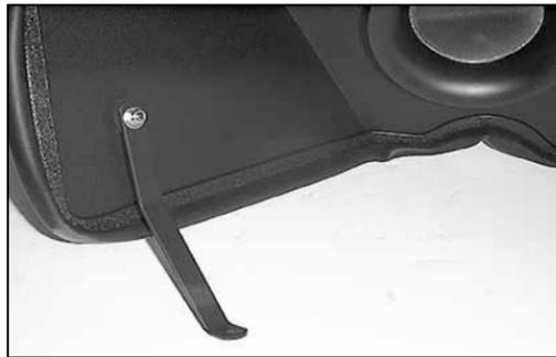
15. Attach the bracket assembly to the heat shield using the hardware provided.
