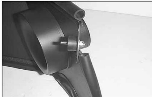
18. Attach a rubber mounted stud to the heat shield using the hardware provided.
