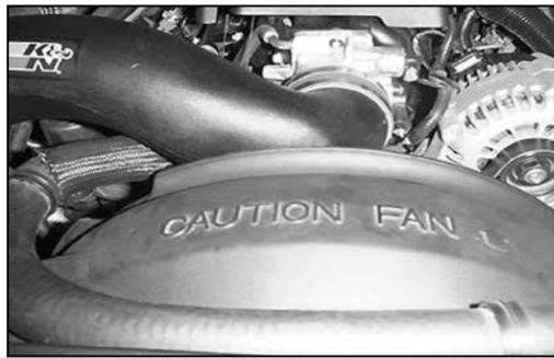
31. Due to production tolerances it may be necessary to mark the fan shroud as indicated, remove the intake tube and trim the fan shroud.
