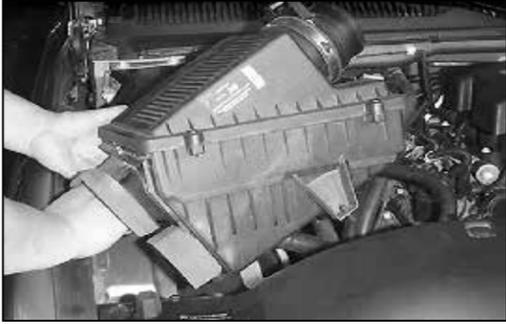
8. Pull firmly upward and remove the airbox.
