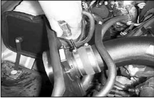
26. Align the intake tube with the mass air sensor and tighten the hose clamp on the silicone hose at the mass air sensor.
