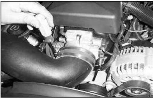
25. Install the intake tube and tighten the hose clamp on the silicone hose at the throttle body.
