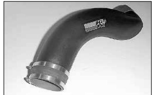
24. Install the 3.75"ID silicone hose (08631) onto the intake tube.
