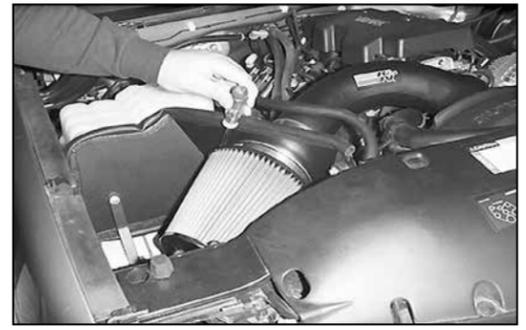
32. Install the air filter and secure with hose clamp.
