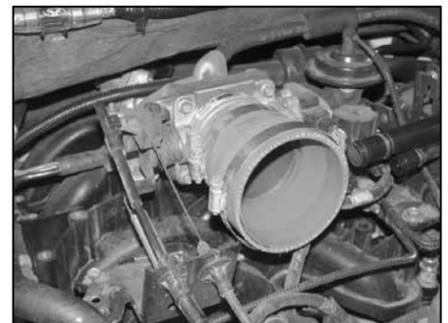
23. Using the provided hose clamp, attach the silicone hose (08724) to the throttle body.
