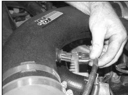
31. Reconnect the air temp. sensor electrical connection.
