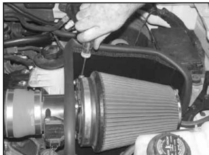
32. Install the K&N® air filter onto the mass air adapter and secure it with the provided hose clamp.
