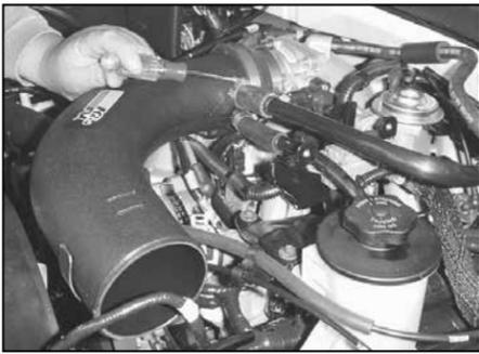
25. On models with 5.4L engines, install the idle air control and crank case vent hose onto the appropriate fittings on the K&N® intake tube, secure with the hose clamps provided.
