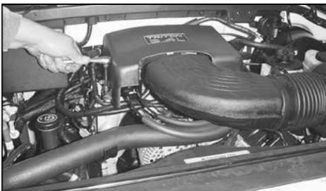
2. Loosen and remove the three bolts that retain the throttle body cover, then remove the cover.
