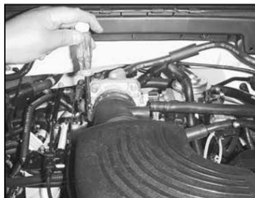
5. Loosen the hose clamp on the stock intake tube at the throttle body.
