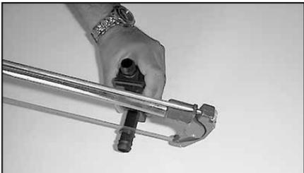
26. On models equipped with 4.6L engines: In some insulated instances where a whistling noise may exist, do as follows. Cut the flange of the air bypass valve just past the last barb. Reinstall the air bypass valve, attaching it to the appropriate fitting on the intake tube using the 5/8" id hose and provided hose clamps.
