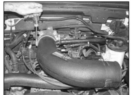
24. Install the K&N® intake tube onto the throttle body and tighten the hose clamp.
