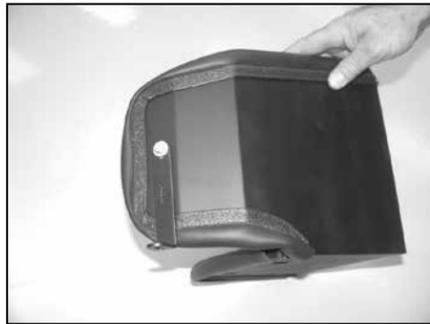
16. Install the provided "L" bracket (070952) onto the heat shield as shown.
