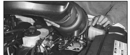
6. Detach the stock intake tube from the throttle body and lift up on the air cleaner assembly to release it from its retaining grommets.
