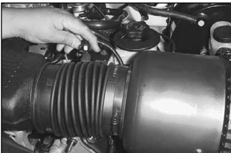
3. Disconnect the air temperature sensor electrical connection.
