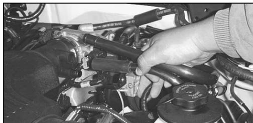
4b. On models with 5.4L engines, detach the idle air control and crank case vent hose from the stock intake tube.
