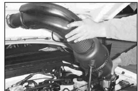
8. Remove the entire stock air intake assembly from the vehicle.
