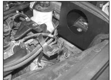
22. Install the saddle bracket assembly onto the protruding stud as shown, secure into place using the provided hardware.
