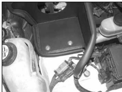
18a. On vehicles not equipped with cruise control, set the heat shield into position on the air filter mounting bracket and then secure the heat shield with the provided hardware as shown.
