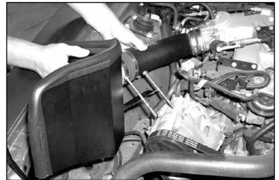
23. Slide the K&N intake assembly into the silicone hose on the throttle body as shown.
