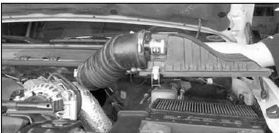
3. Loosen the hose clamp at the intake manifold. Release the clips from airbox top then remove complete upper intake.
