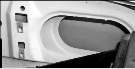
12. Vehicles that are not equipped with the fuse box, use the two upper mounting clips that were removed in step 7 and install onto inner fender wall.
