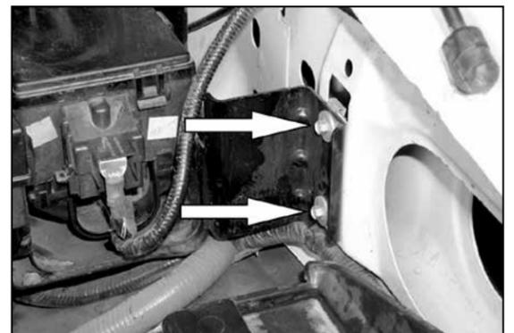
11. Remove the two bolts that retain the fuse box mounting bracket as shown.
