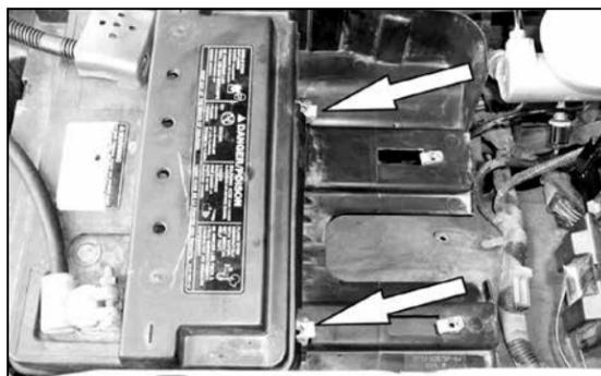
7. Remove the two upper airbox mounting clips.
