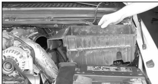
6. Then remove the stock airbox base from vehicle. **NOTE: K&N Engineering, Inc., recommends that customers do not discard factory air intake.**
