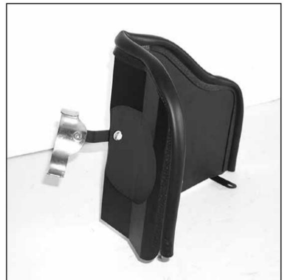
10. Install saddle bracket assembly onto heat shield as shown. Do not tighten completely.
