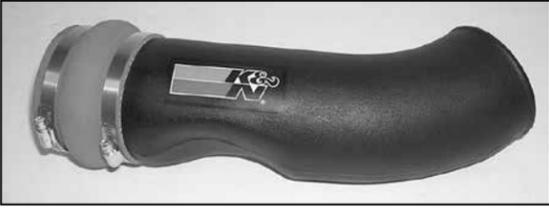
13. Install the silicone hump hose and hose clamps onto the K&N® intake tube as shown.
