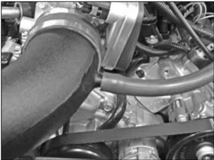
31. Install the provided crank case vent hose onto the valve cover and then onto the intake tube as shown.
