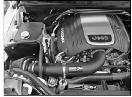
37. Reconnect the vehicle's negative battery cable. Double check to make sure everything is tight and properly positioned before starting the vehicle.
