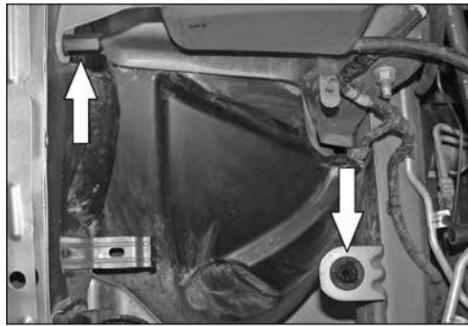
20. Remove the coolant reservoir-retaining nut and air box mounting grommet shown.
