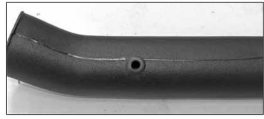
26. Install the provided grommet into the intake tube as shown.
