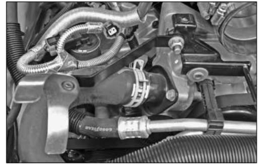
25. Install the tube mounting bracket assembly onto the plenum mount and secure with the factory nut removed in step #23.
