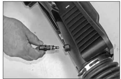
27. Rotate the air temperature sensor counter clockwise and remove the sensor from the stock intake plenum as shown.
