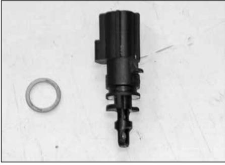
28. Remove the rubber sealing "O" ring from the air temperature sensor as shown.
