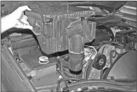
14. Lift the lower air box and remove it from the vehicle as shown.
