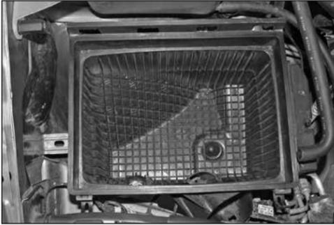
13. Remove the air box mounting bolt shown.
