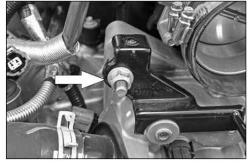
23. Remove the nut, which secures the intake plenum-mount shown.
