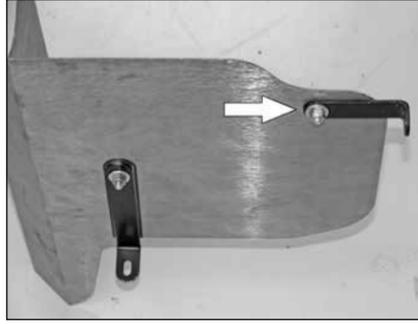
17. Install the small "L" bracket (07158) onto the heat shield as shown with the provided hardware.
