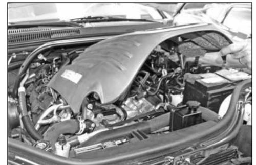
7. Remove the engine cover from the engine as shown.
