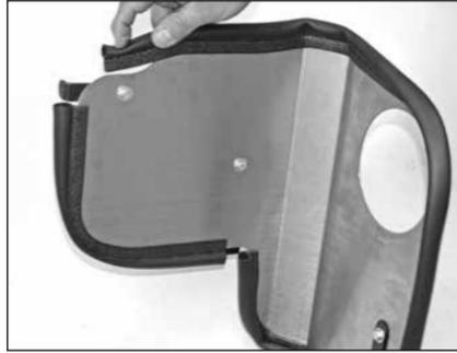
19. Install the long edge trim onto the heat shield assembly as shown.
