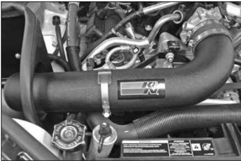
30. Install the intake tube into the silicone hose at the throttle body and onto the saddle clamp, then secure with the provided hose clamps.
