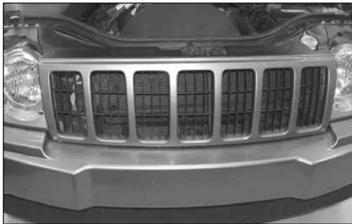
36. Reinstall the grill assembly with the factory retaining clips removed in step #5.
