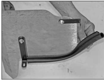
18. Install the short edge trim onto the heat shield assembly as shown.
