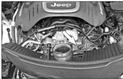
5. Pull the intake plenum off the throttle body and rotate forward, then disconnect the crank case vent hose from the tube attached to the intake plenum. **NOTE: Do not completely remove the intake plenum at this time.**
