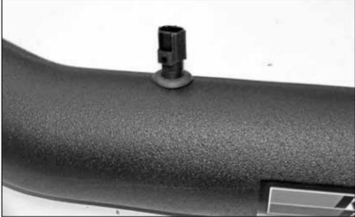
29. Install the air temperature sensor into the intake tube as shown.
