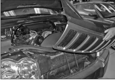
11. Remove the six grill retaining clips from the grill, then tilt the grill forward and lift to remove from the vehicle.
