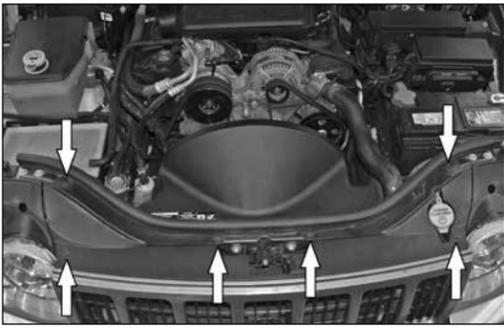
10. Using a small screwdriver, release the center holding pins in the six grill retaining clips shown.
