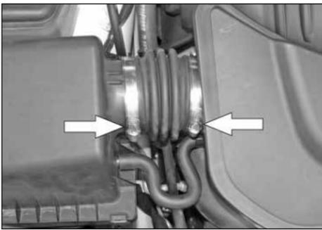
2. Loosen the hose clamp, which secures the stock intake tube to the intake plenum, and disconnect the crank case vent hose from the air box lid.
