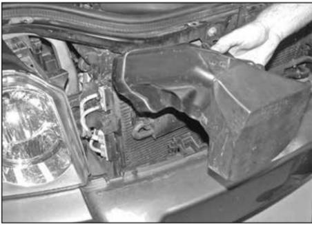
12. Pull the fresh air duct forward to disconnect it from the air box and then remove it from the vehicle.
