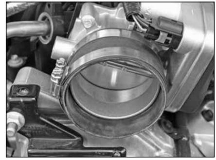
22. Install the silicone hose (08630) onto the throttle body and secure with the hose clamp provided.
