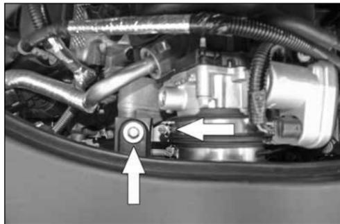
4. Remove the intake plenum-mounting bolt and loosen the intake plenum hose clamp at the throttle body.
