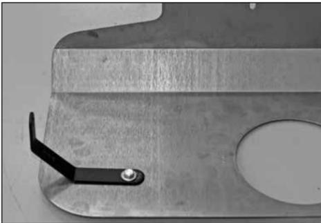
15. Install the supplied "C" bracket (07171) onto the heat shield as shown with the provided hardware. **NOTE: Due to manufacturing tolerances, it may be necessary to use the provided spacer and longer bolt to attach the mounting bracket to the heat shield. This will enable the mounting bracket to align with the longer air box mounting brackets on some vehicles.**
