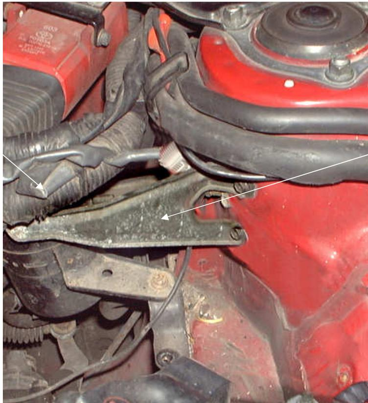
2. Remove the two securing bolts from the side of the suspension turret and remove the harness mounting bracket.
