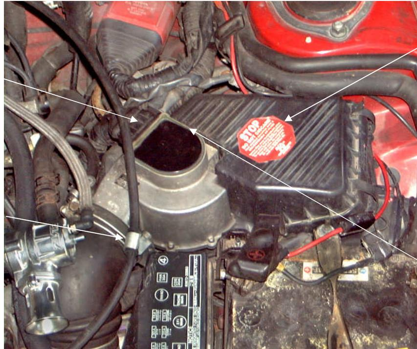
3. Unclip and remove the air box lid assembly.
