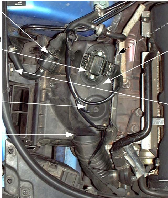
**5.** Remove the 4 screws securing the heat shield to the air box assembly
