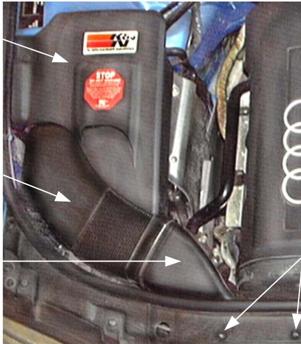
**3.** Remove the intake scoop from the slam panel by removing the 2 securing screws.
