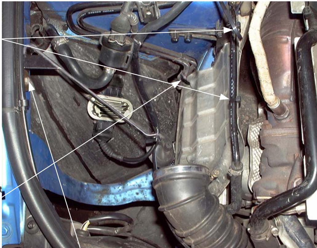
1. Attach the amplifier to the hole in the side of the mounting bracket using one of the original screws in the amplifier.
