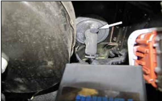
8. Poke a small hole in the existing firewall grommet and feed the boost control knob harness through the grommet from the inside of the vehicle. Connect the control knob harness to the pigtail connected to the module and secure with the provided tie wraps.
