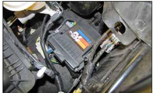
6. Mount the boost module in a suitable location such as under the brake master cylinder as shown using the provided tie wraps.
