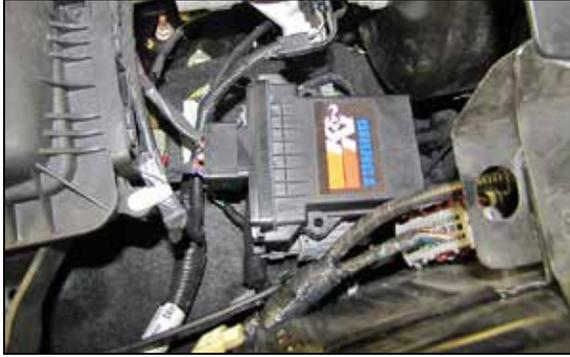
7. Connect the boost harness to the module and secure with the locking bolt.
