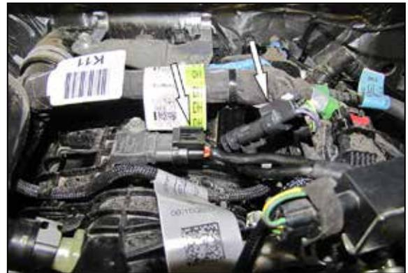
5. Connect the K&N® harness to the MAP sensor and to the factory harness. Route the K&N® harness towards the driver's side inner fender. Secure the harness with the provided tie wraps. Reinstall the decorative engine cover.
