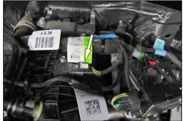
4. Disconnect the MAP sensor electrical connection at the rear of the intake manifold.
