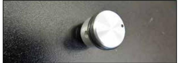
9. Find a suitable location to mount the sensitivity knob, drill a  $\frac{1}{4}$ "id hole, remove the knob and install the rheostat then reinstall the knob.
